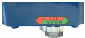
**Please Note:** Because the actuator does not have mechanical limit stops, be careful not to rotate past the valves full open or closed position.
