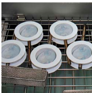
Cleansing the parts with ultrapure water
