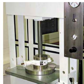
Tightness test with HP nitrogen
