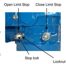
**Please Note:** Do not set the actuator position limit switches to drive into the mechanical stops. Permanent damage will occur if the motor is allowed to repeatedly stall into the end stops.
